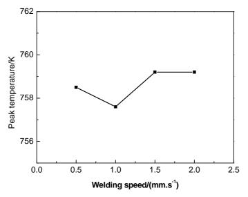
Fig. 3. Effect of different welding speed on peak temperature
